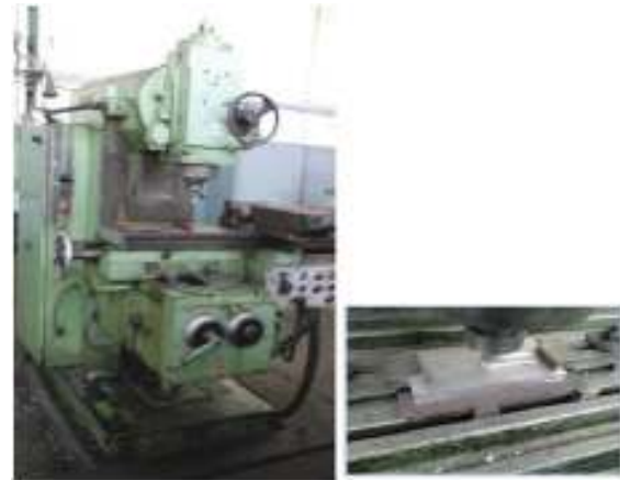
Figure 2: Friction Stir Process Machine and Component
