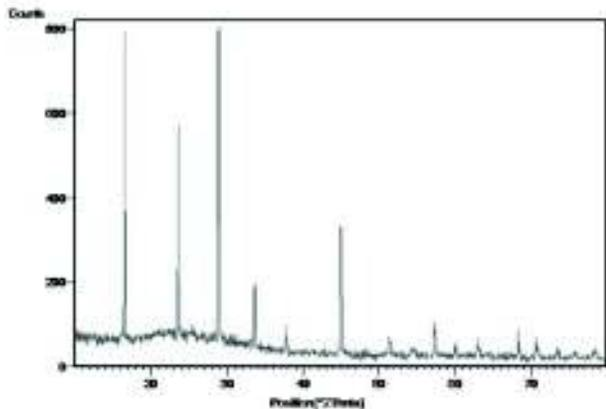
Figure 2 : Powder XRD Pattern of L-Proline Doped ADP
