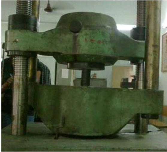
Figure 12 : Static Testing of Composite Spring on UTM
