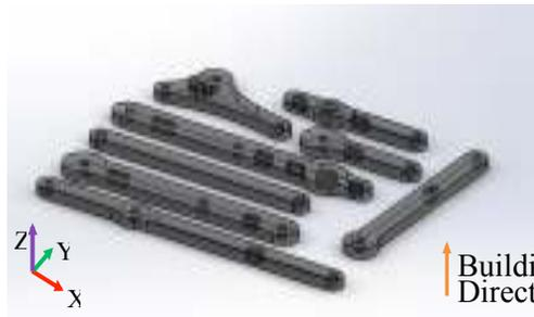
Fig 2(b) 3D printing orientation
