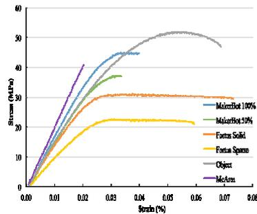
Figure 6. Stress-strain curve comparison
