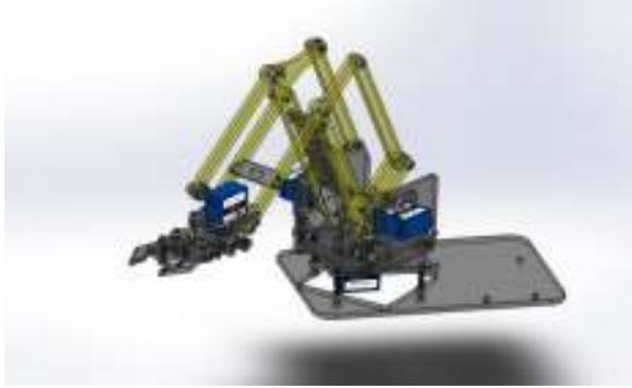
Fig 1.3D model of MeArm
