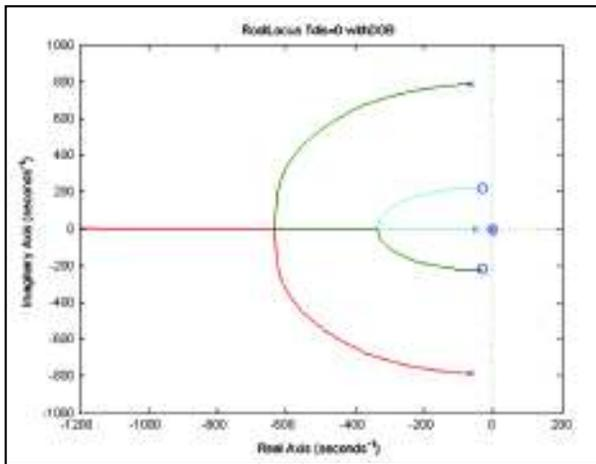
Figure 7 : Root locus plot for  $T_{dis}=0$ , with DOB
