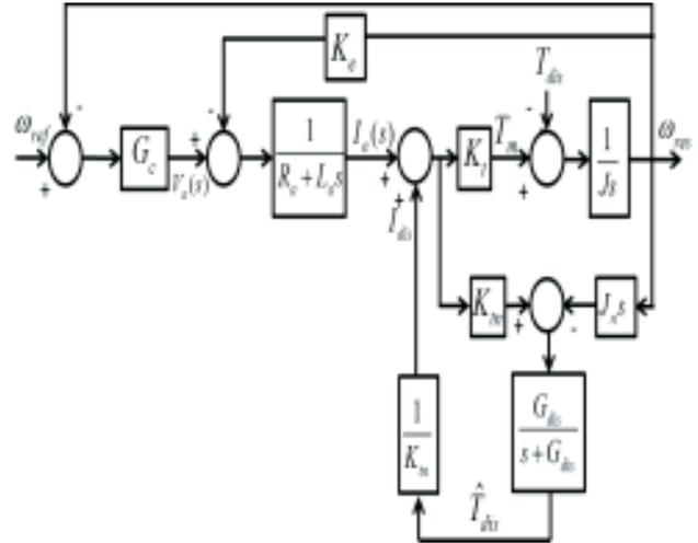
Figure 5: PID based velocity controller with DOB
