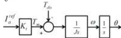
**Figure 3: Block diagram of the motor with disturbance**
