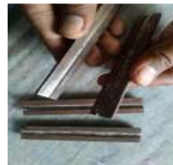
Figure 5. steel casing for the ends of the test specimens The bars thus made is mounted on to the UTM and the Tension test is carried out.
