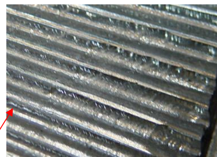
Figure 9. Iso parametric machining surface and its measuring results (in mm). It can be seen chatter marks in some area of the surface. Shows the measuring direction.
