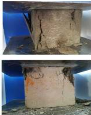
Fig.9 Failure of the cube under compression
