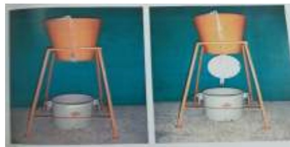
Fig.1 Test set up for determining the packing density of aggregates.
