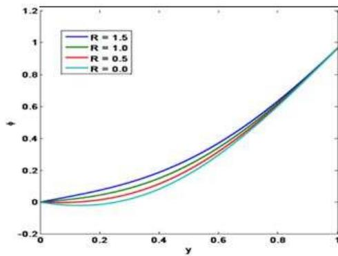
Figure 10: Concentration profile for various suction parameter (R) [Pe = 1, Pr = 0.5, Sr = 0.5,  $\alpha = 5$ ,  $x = 1$ ,  $\varepsilon = 0.02$ ,  $\lambda = 0.4$ ]
