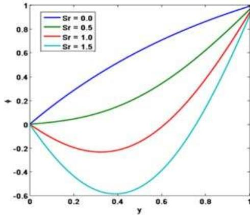
Figure 9: Concentration profile for various Soret number (Sr) [Pe = 1, Pr = 0.5, R = 0.5,  $\alpha = 5$ ,  $x = 1$ ,  $\varepsilon = 0.02$ ,  $\lambda = 0.4$ ]
