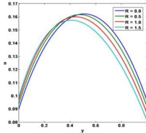
**Figure 3: Velocity profile for various suction parameter ( $R$ ) [ $c = -1, M = 2, \gamma = 0.3, x = 1, \epsilon = 0.02, \lambda = 0.4, m = 0.5, \theta = 60^\circ$ ]**
