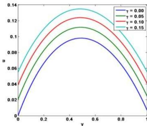
**Figure 2: Velocity profile for various slip parameter ( $\gamma$ ) [ $c = -1, M = 2, R = 0.5, x = 1, \epsilon = 0.02, \lambda = 0.4, m = 0.5, \theta = 60^\circ$ ]**
