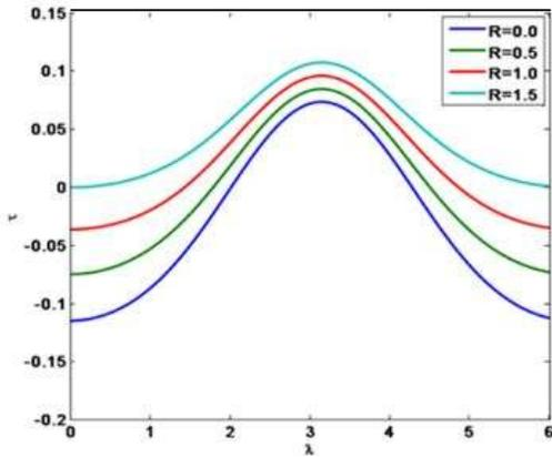
**Figure 13: Skin friction for various suction parameter (R) at wavy wall**
