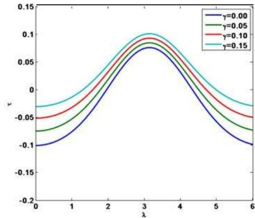
**Figure 15: Skin friction for various slip parameter ( $\gamma$ ) at wavy wall [ $c = -1, M = 2, x = 1.0, \varepsilon = 0.02, r = 5, m = 0.5, \theta = 60^\circ$ ]**
