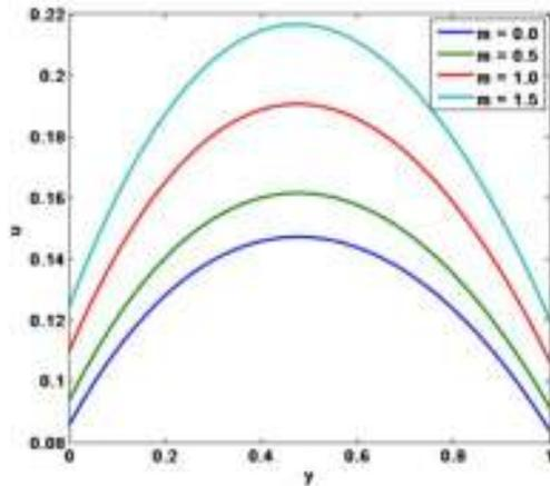
**Figure 5: Velocity profile for various Hall parameter ( $m$ ) [ $c = -1, \gamma = 0.3, R = 0.5, x = 1, \varepsilon = 0.02, \lambda = 0.4, M = 2, \theta = 60^\circ$ ]**
