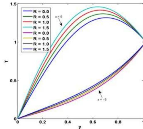
**Figure 7: Temperature profile for various suction parameter ( $R$ ) [ $Pr = 0.5, x = 1, \varepsilon = 0.02, \lambda = 0.4$ ]**
