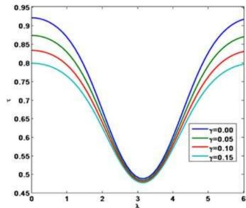
**Figure 16: Skin friction for various slip parameter ( $\gamma$ ) at flat wall [ $c = -1, M = 2, x = 1, \varepsilon = 0.02, R = 0.5, m = 0.5, \theta = 60^\circ$ ]**
