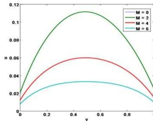
**Figure 4: Velocity profile for various Hartmann number ( $M$ ) [ $c = -1, \gamma = 0.05, R = 0.5, x = 1, \epsilon = 0.02, \lambda = 0.4, m = 0.5, \theta = 60^\circ$ ]**
