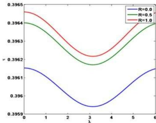
**Figure 14: Skin friction for various suction parameter (R) at flat wall [ $c = -1, M=2, x=1.0, \varepsilon = 0.02, r=5, m=0.5, \theta = 60^\circ$ ]**
