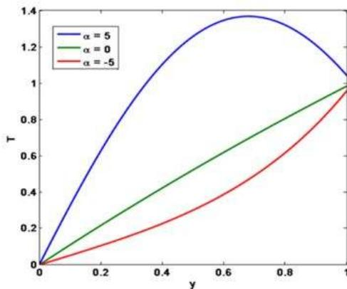
**Figure 6: Temperature profile for various heat source parameter ( $\alpha$ ) [ $Pr = 0.5, R = 0.5, x = 1, \varepsilon = 0.02, \lambda = 0.4$ ]**
