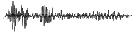
A Graph Shows Response for El Centro Ground Motion in X-direction for framed structure
