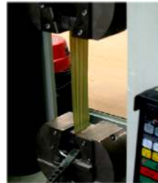
Fig. 4: The universal testing machine used for tensile testing of polyethylene
