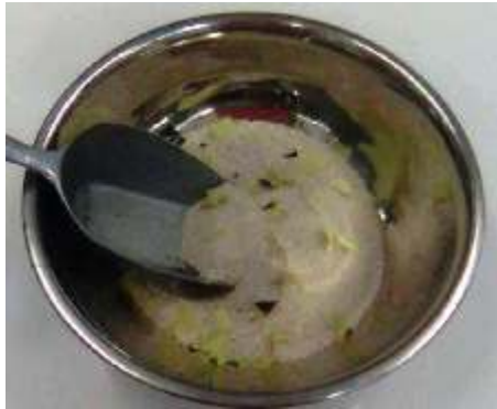
Fig. 5: Randomly mixed sand-plastic composite for testing
