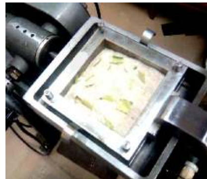
Fig. 7: Soil-plastic composite sample placed in shear box for strength testing
