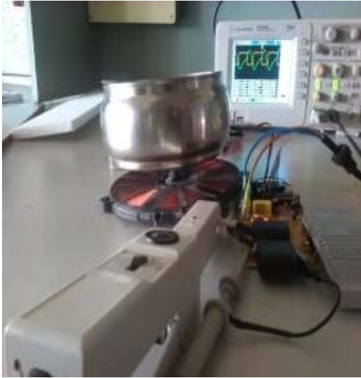
Fig.7.1. Experimental setup of Circuit with the load Vessel
