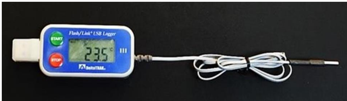
Figure 3: Data recorder with temperature sensor (Credit: Lauren Douma, UF)
