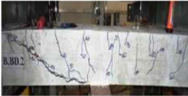
The shear failure of slab B.BD.2
