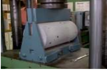
Fig: 4.4 showing test by Split Tensile Strength
