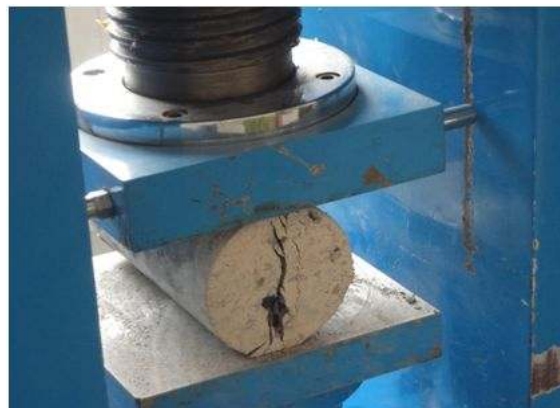
Figure 5: Split Tensile Test
