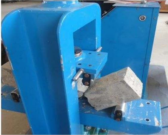
Figure 6: Flexural Strength Test
