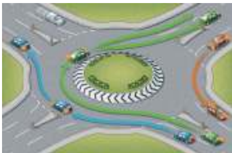
Fig. 5 Typical Example Roundabout
