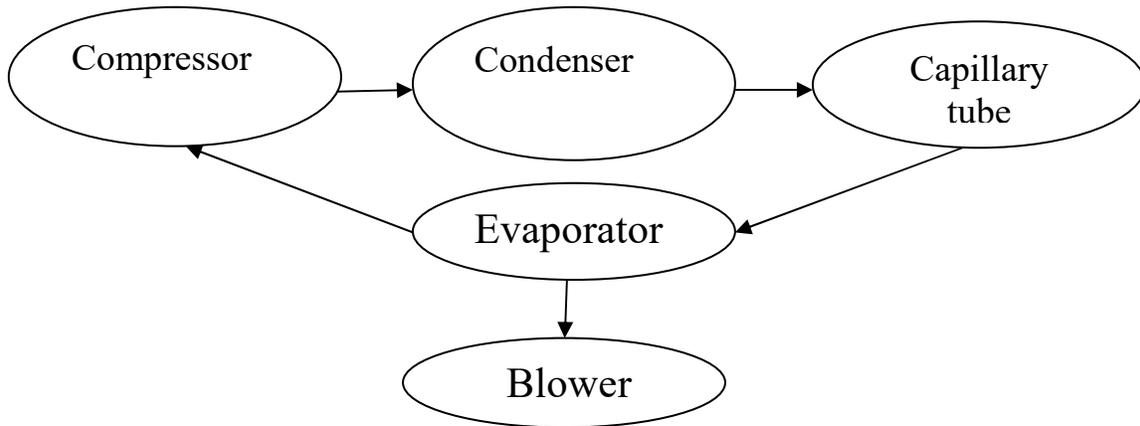
**Figure 1: Line diagram of designed cooling device**
