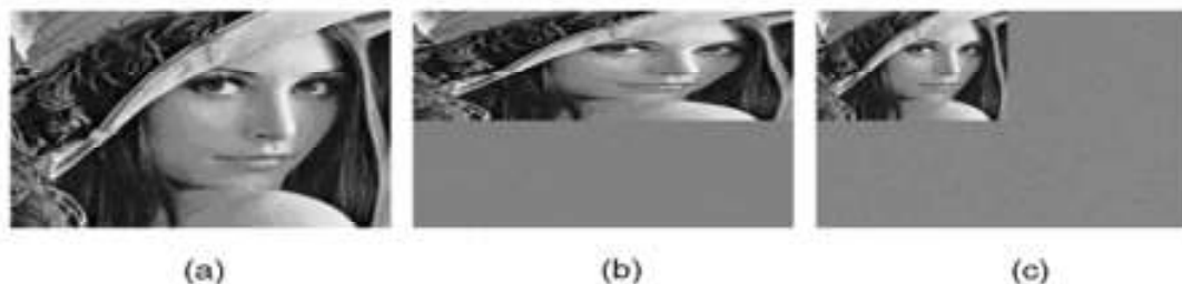
Figure 9: DWT for Lena image (a) Original Image (b) Output image after the 1-D applied on column input (c) Output image after the second 1-D applied on row input
