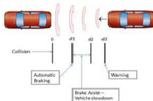
There aren't technologies to prevent accidents. But they have introduced sensors that would detect any obstacles. Besides this it also gives an alert to the driver. In this work we are enhancing the existing work by introducing automatic brakes with distance adjustment, which would get its input
