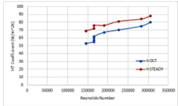
Fig 4.Relation between Reynolds number and heat transfer coefficient
