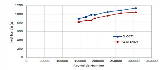
Fig 5. Relation between Reynolds number and Heat Transfer
