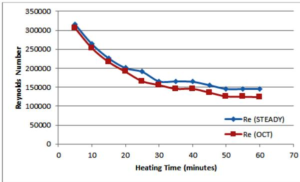
Fig 2. The relation between the heating time and Reynolds number
