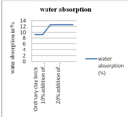
Figure 3: Water Absorption
