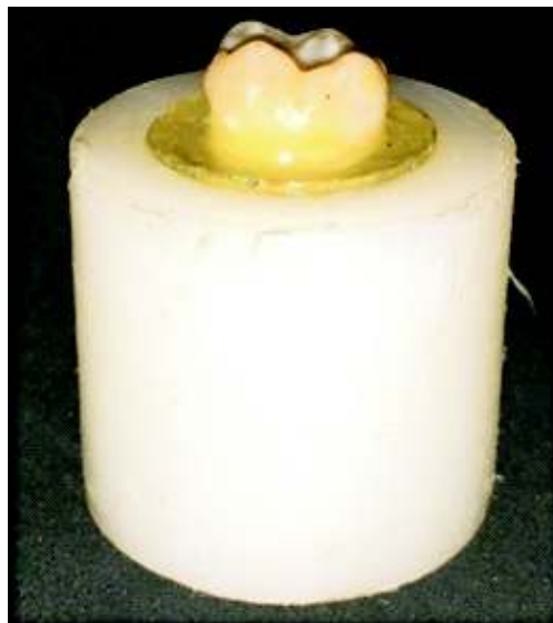
Figure 1 : Teeth Mounted in Epoxy Resin Blocks Using Custom Made Teflon Mold
