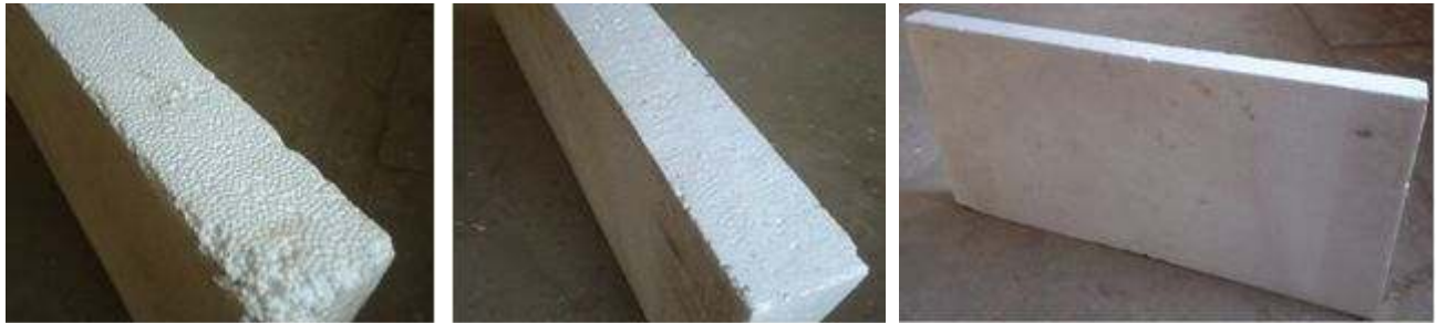
Figure 2: Typical 100 mm 60 mm thick EPS sheets
