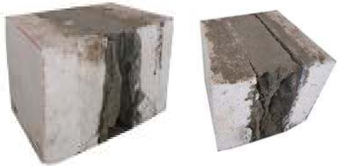
Figure 5: Tested ICF blocks with 100 and 50 mm thick EPS
