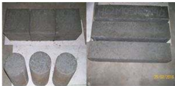
Figure 2: Concrete samples after 24 hrs of casting
