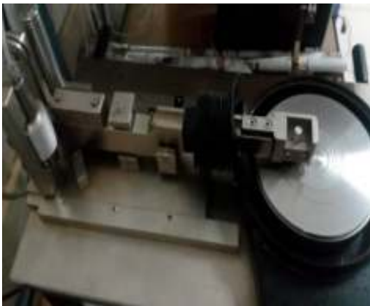
Fig.3 - Schematic of pin-on-disk apparatus
