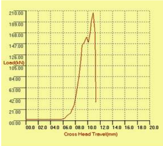
Figure 9: 60mm Thick Plain Concrete
