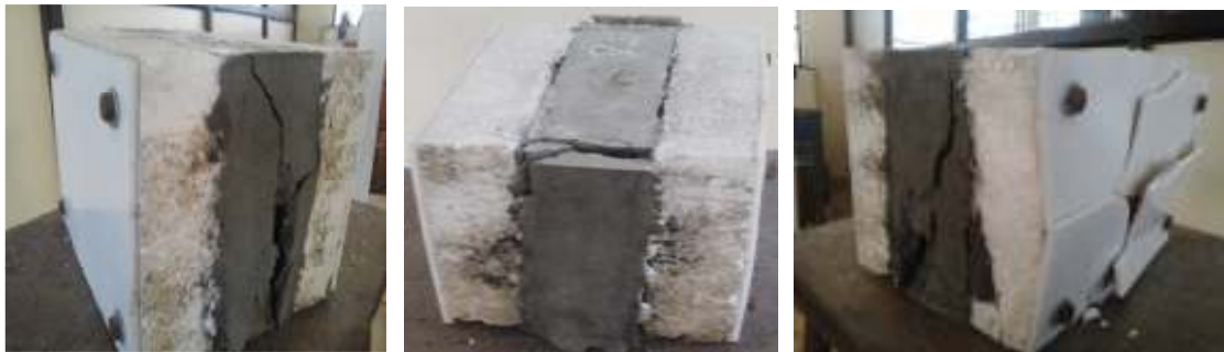
Figure 8: Typical Tested ICF Blocks with Polypropylene sheets
