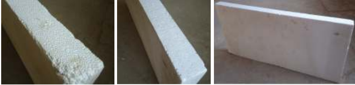
Figure 3: Typical 100 mm 60 mm thick EPS sheets
