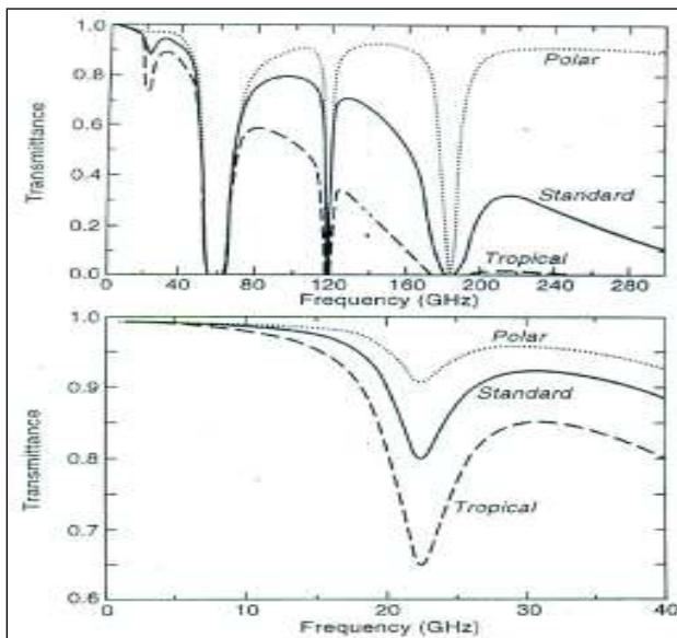
**Figure 4:** The transmittance at normal incidence angle for cloud-free subpolar (dotted line), midlatitude (solid line) and tropical (dashed line) atmospheres as a function of frequency. The frequency range 0 to 300 GHz is shown in the upper panel and an enlargement for the frequency range 0 to 40 GHz is shown in the lower panel
