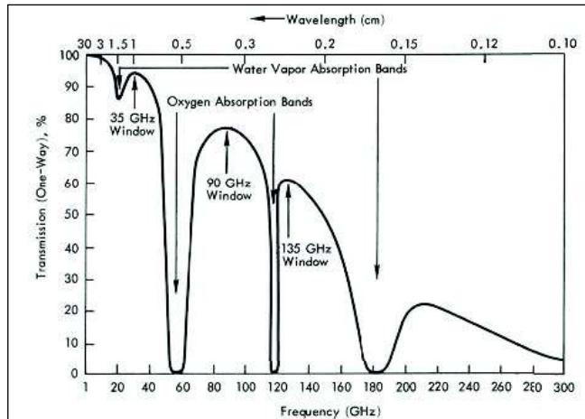
**Figure 1: Percentage transmission of microwave through the earth's atmosphere, along the vertical direction, under clear sky conditions**
