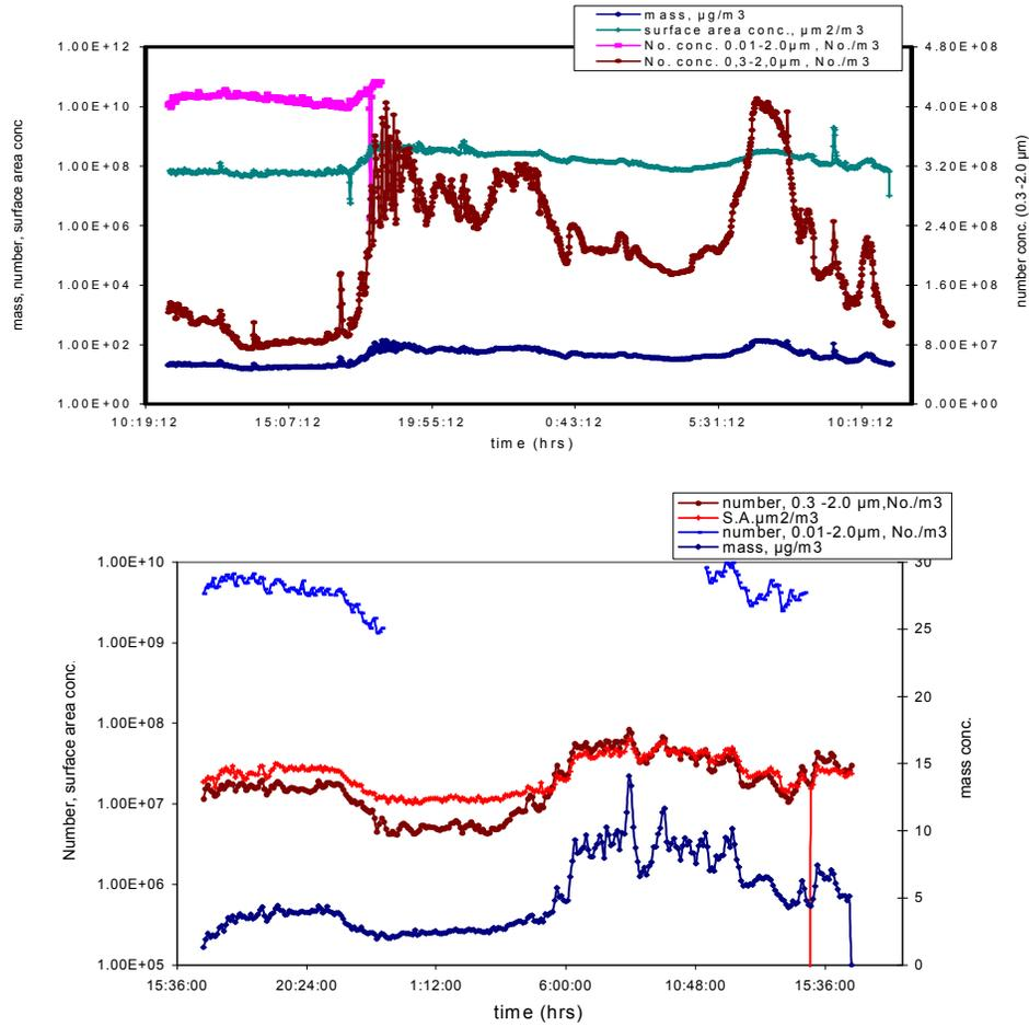
Fig. 3: Plot showing concentration levels over a day at outdoor city peripheral sites: NC data is sparse due to the weakening of alcohol cartridge in CPC
