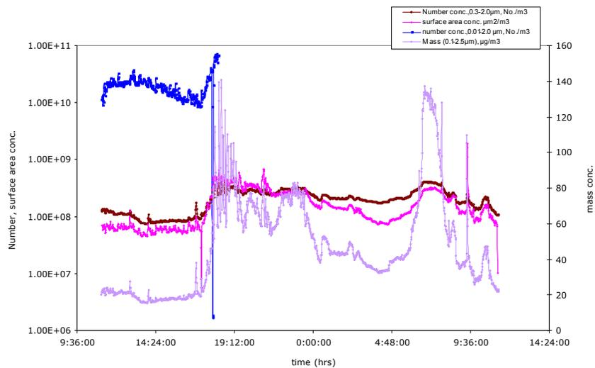
**Fig. 4:** Plot showing concentration levels over a day at an outdoor city centre site: CPC data is sparse due to the weakening of alcohol cartridge, CPC data showing a sudden dip due to the weakening of cartridge
