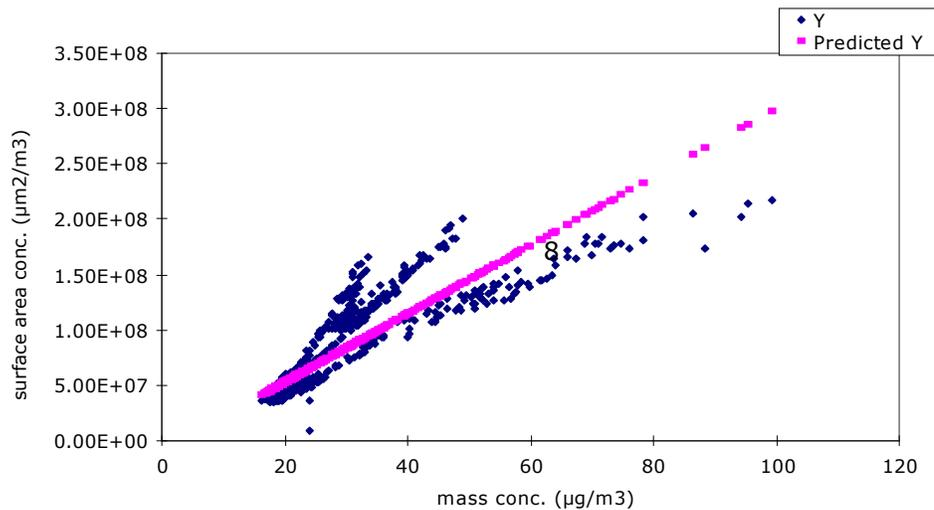
**Fig. 2: Regression analysis plot for MC (100 – 2500 nm) and SAC (10 nm – 2000 nm) at a city peripheral outdoor site. Interestingly, three clear distinct relations can be seen  $r^2 = 0.77$ , Regression equation:  $Y = (3.09E+6)x - (0.97E+07)$**
