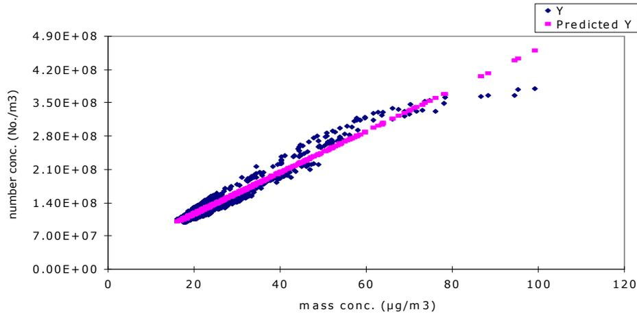
**Fig. 1. Regression analysis plot for MC (100 – 2500 nm) and NC1 (300 - 2000 nm) at a city peripheral outdoor site.  $r^2 = 0.94$ , Regression equation:  $Y = (4.34E+06)x + 2.89E+07$**
