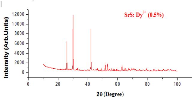
**Figure 1: XRD of pure SrS: Dy<sup>3+</sup> (0.5 mol %).**
