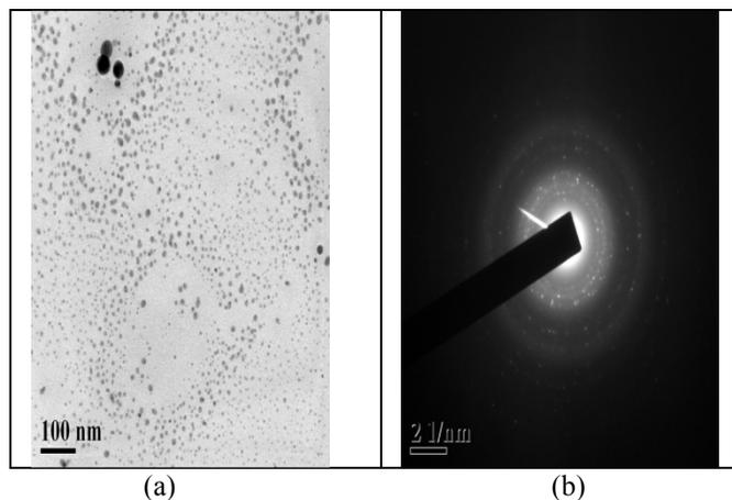
Fig. 4: (a) HRTEM image of SrS:  $Dy^{3+}$  (0.5mol %) phosphor (b) SAED image of SrS:  $Dy^{3+}$  (0.5mol %) phosphor.
