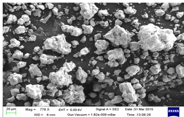
**Fig. 2. FESEM image of SrS: Dy<sup>3+</sup> (0.5mol %) phosphor.** The EDX qualitative and quantitative elemental analysis of SrS: Dy<sup>3+</sup> phosphor sample is depicted in fig. 3. The result of EDX studies verifies the presence of strontium (Sr), sulphur (S) and dysprosium (Dy) in the prepared sample. Further, it is observed that the distribution of the elements is fairly uniform. Qualitative analysis of prepared sample was shown in table 1.
