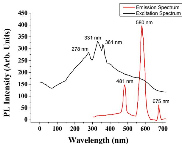
Fig. 5: PL of SrS:  $Dy^{3+}$  (0.5mol %) phosphor
