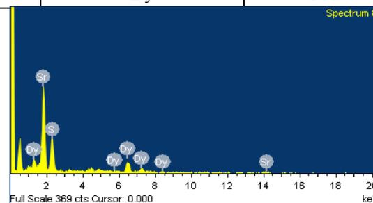
**Fig.3: EDX spectra of SrS: Dy<sup>3+</sup> (0.5mol %) phosphor**
