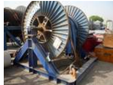
Figure 1: Typical example of drill line frame (courtesy by Sedco Engineers Pvt. Ltd.)
