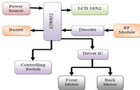
Figure 3.4 Receiver Section
