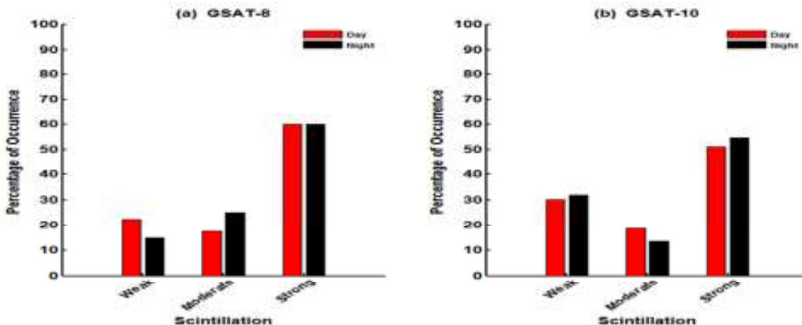
Figure 3: Percentage of occurrence of weak, moderate, strong day and night time amplitude scintillation events during equinox of 2014 for (a) GSAT-8 and (b) GSAT-10.
