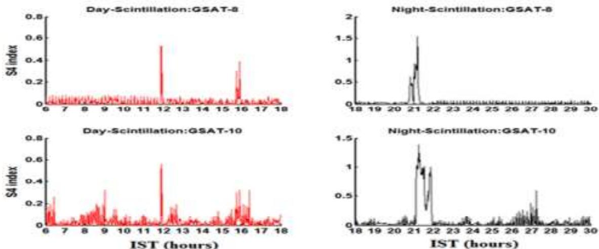
Figure 1: The typical examples of day time and night time amplitude scintillations of GSAT-8 and GSAT-10 on 05<sup>th</sup> March 2014.
