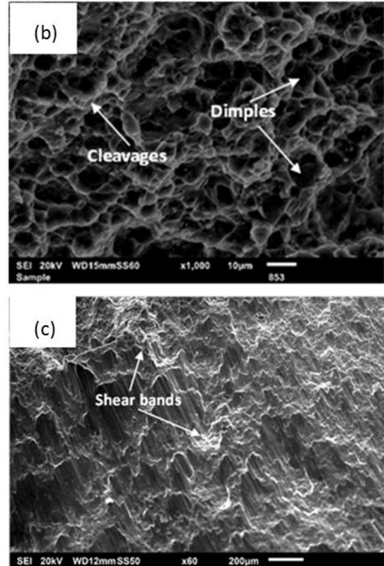
**Figure 2: (a) Tension compression curves showing the yield asymmetry trend; (b) Tensile and (c) Compressive fractographies of the Mg-3Gd-0.4Ce alloy.**
