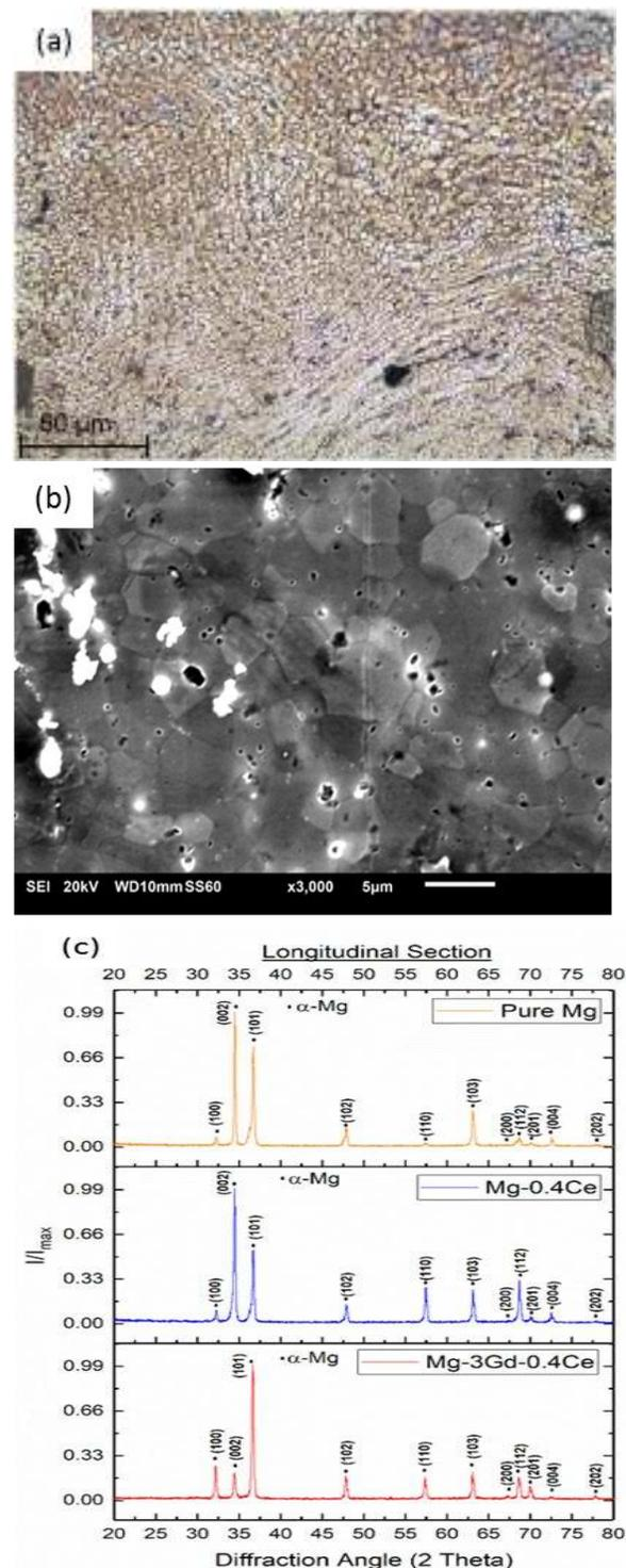
**Figure 1: (a) Optical micrograph of Mg-3Gd-0.4Ce alloy; (b) Microstructure of Mg-3Gd-0.4Ce alloy; (c) XRD results of extruded samples along longitudinal section.**
