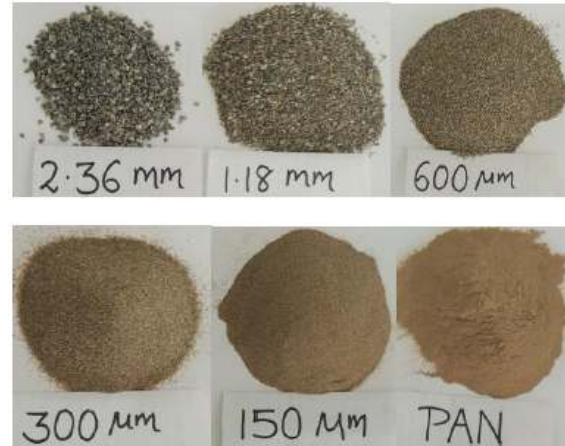
Figure 1: Residues of crusher dust passing through different Sieves
