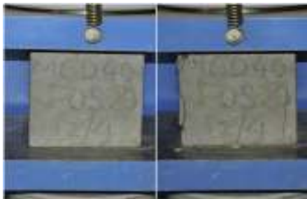
Figure 4: Cube specimen before and after failure
