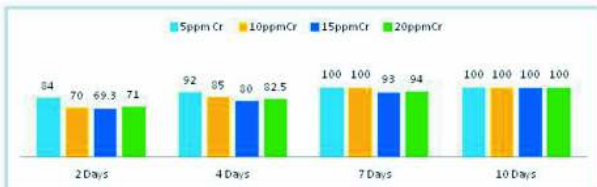
Fig. - 1 % absorption of Chromium by 1500 g of Eichhornia crassipes over different incubation periods.
