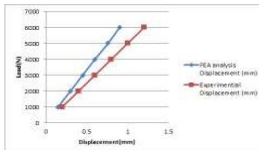
**Figure 16: Load versus Displacement graph for Model M1 Scaffold Structure made with PLA by FEA and Compression test**
