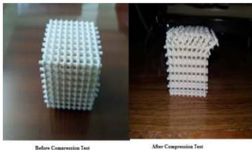
**Fig.15: Shape of Model 2 scaffold structure before and after the compression test**
