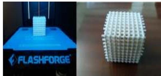
**Figure 13: Fabricated model of Solid Sphere Interconnected Rod**
