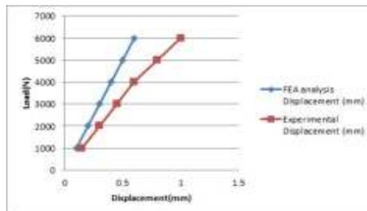
**Figure 17: Load versus Displacement graph for Model M2 Scaffold Structure made with PLA by FEA and Compression test**
