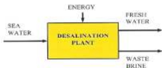
Fig (1).Main inputs and outputs in a desalination process. Source: CLAYTON (2007)
