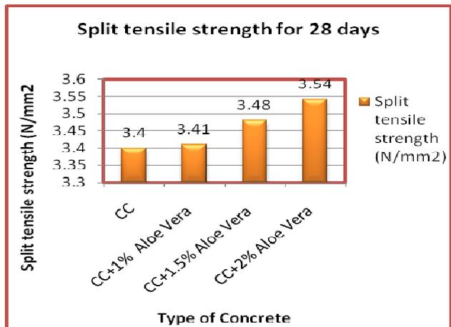
The split tensile strength was found higher in concrete added with natural admixture. From the above result we can conclude that the self-curing showed 4% increase in split tensile strength when compared to conventional concrete.
